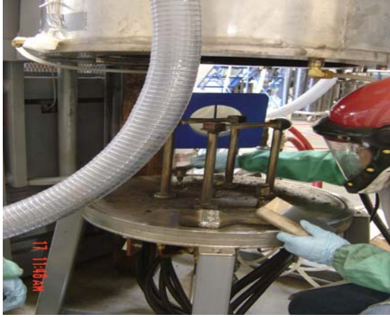
Figure 3: Typical location of fume extractor and production operator during reactor cleanout activities (filter-based air sampling devices located in upper left corner of photo on left)
