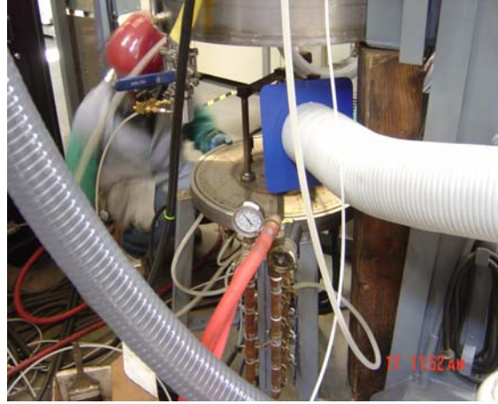
Figure 3: Typical location of fume extractor and production operator during reactor cleanout activities (filter-based air sampling devices located in upper left corner of photo on left)
