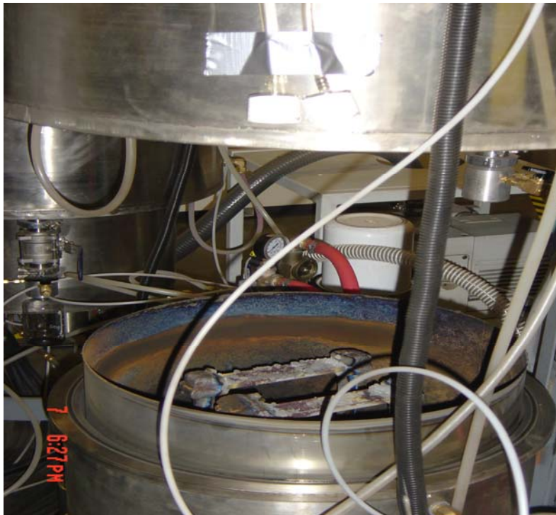
Figure 2: Reactor cleanout process with no fume extractor (LEV)
